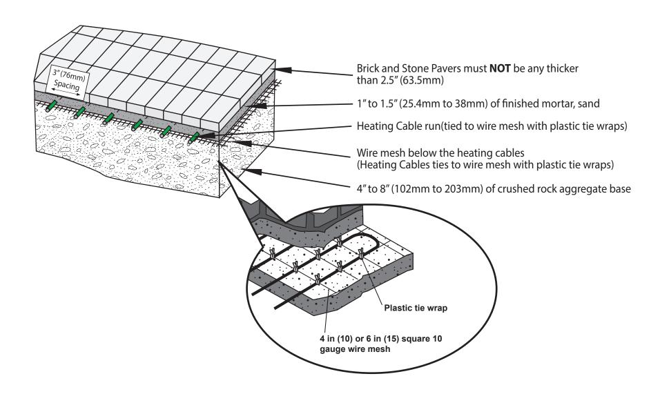
Note: Cables may be tied to reinforcement type mesh and then the mesh should be staked down to the base/crushed rock aggregate.
