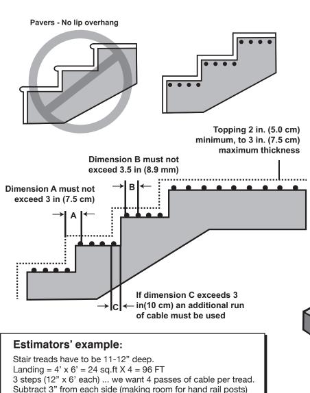
Stair treads have to be 11-12" deep. Landing = 4' x 6' = 24 sq.ft X 4 = 96 FT 3 steps (12" x 6' each) ... we want 4 passes of cable per tread. Subtract 3" from each side (making room for hand rail posts) 5.5' X 4 = 22 FT plus 3 FT = 25 FT per tread 3 FT is the amount needed for curves and tread riser. Solution: 96 FT + 25 FT + 25 FT =  $\boxed{171 \text{ FT}}$
