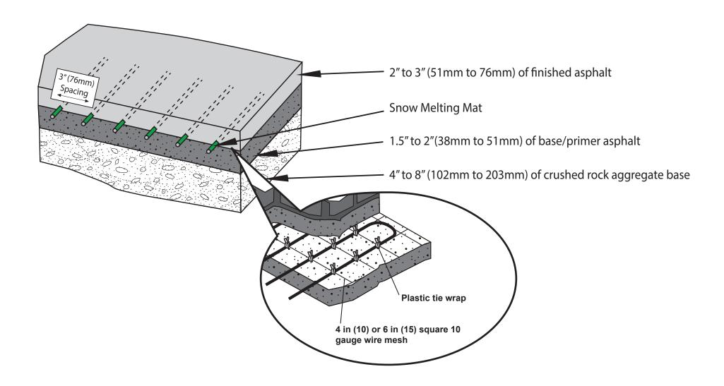
Note: Cables may be tied to reinforcement type mesh and then the mesh should be staked down to the base/primer pour.
