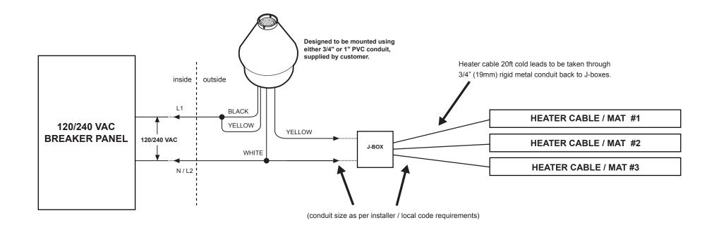
INSTALL IN ACCORDANCE WITH THE REQUIREMENTS OF ALL APPLICABLE ELECTRICAL AND BUILDING CODES AND REGULATIONS. ENSURE THAT ALL CONDUIT/CABLE TERMINATIONS ARE WATERTIGHT.
