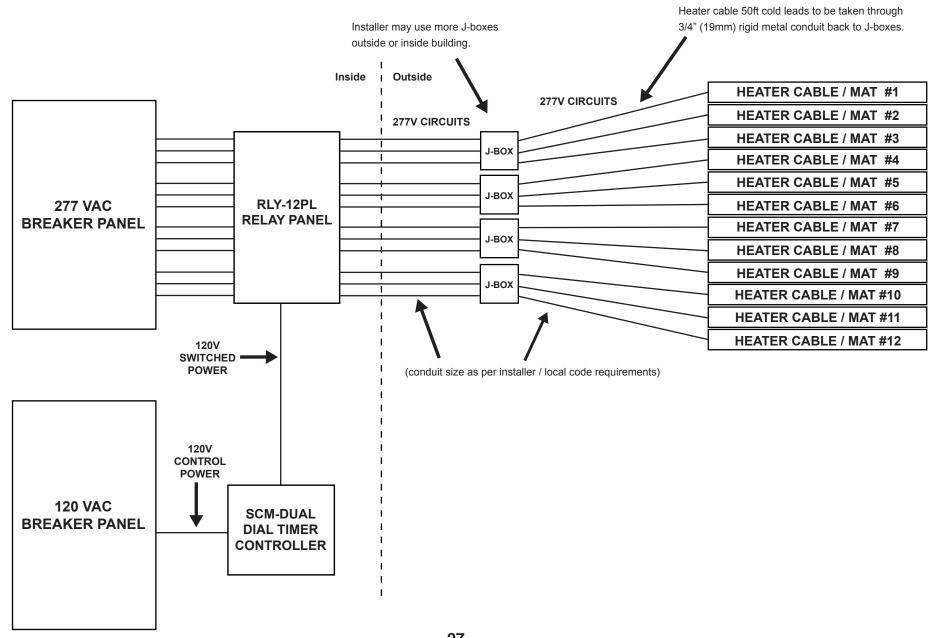
**APPENDIX 0:** SNOW MELT DIAGRAM 208V - TYPICAL LINE DIAGRAM (FOR 6 CIRCUITS/CABLES) WITH MANUAL CONTROL
